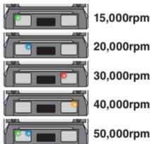
**Commentary** This determines the motor rpm at which the boost will end. As this rpm value is set higher, boost will operate to a higher speed/rpm point.
