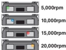
**Commentary** This determines the motor rpm at which the boost will begin to operate. As this rpm value is set lower, boost will operate from a lower speed/rpm point.
