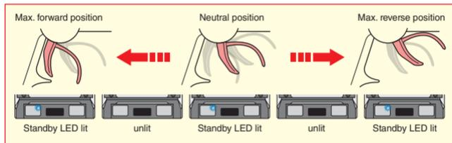
If the standby LED does not follow this lighting pattern, the initial setting was not completed properly. Make sure the throttle related adjustment on the transmitter are initialized and the RX cable is properly connected to the receiver. Then, retry the initial setting procedure.
