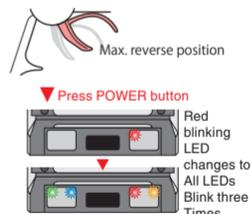
This completes the initial settings for the transmitter positions. The ESC automatically changes to the standby mode (p. 8).
