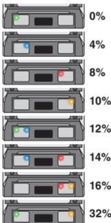
**Commentary** It is the amount of braking force applied when the throttle is returned to neutral. The higher the value = increased braking force
