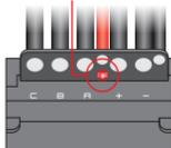
**Important** This function protects only the ESC circuit board when the battery is reversely connected. Capacitors connected to ESC such as Chevalier series are not protected, so be careful when connecting batteries.
