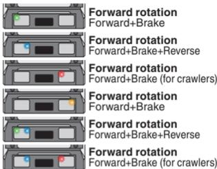
**Commentary** Switched between normal and reverse motor rotation. Regardless of whether the initial settings have been completed properly, the car may go into reverse once the throttle is applied. If this condition occurs, please use Reverse rotation operation mode. The orange LED will be lit in standby mode when Reverse rotation is selected.
