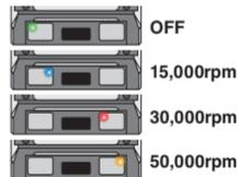
**Commentary** This function limits the output of the motor so that the rpm does not exceed the set value.
